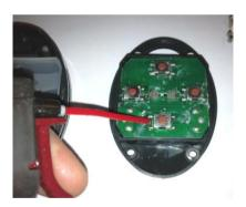
Mount switch board and rubber keyboard
